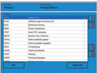
Downtime confirmation on machine terminal
